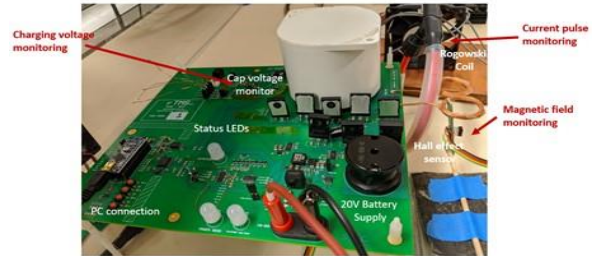
Fig.3: (a) Testbed for rTMS measurement and (b) photo of electronic board and measurement instruments.
