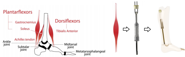
(a) Principal joints and muscles (b) Concept design of bioinspired muscles of the ankle-foot complex [12] spired muscles
