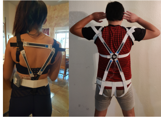
Fig. 1. Left figure shows a triangular configuration with 3 stretch sensors reported in [7]. Right figure shows the new cross configuration with 4 sensors.
