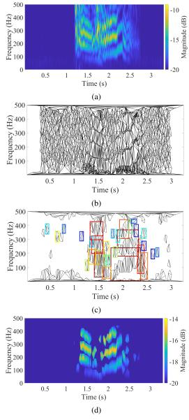
Fig. 4: Noise removal based on the spectogram zeros applied to a single BS.
