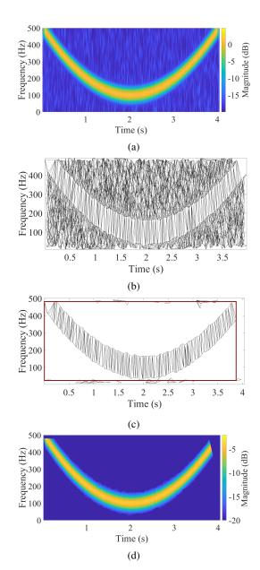
Fig. 1: Stationary noise removal based on the spectogram zeros applied on a noisy quadratic chirp: (a) STFT magnitude, (b) Delaunay triangles whose vertices coincide with zero values, (c) selected domain with large edge length, (d) masked STFT.
