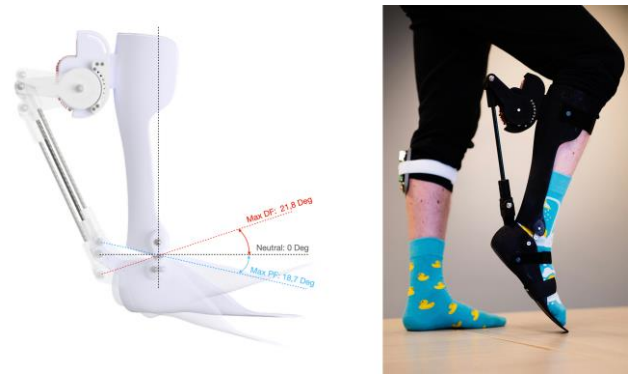
Fig. 6: Left: PAFO assembly with cuffs and actuation system with a 4-bar mechanism Right: Test subject wearing the assembled PAFO prototype
