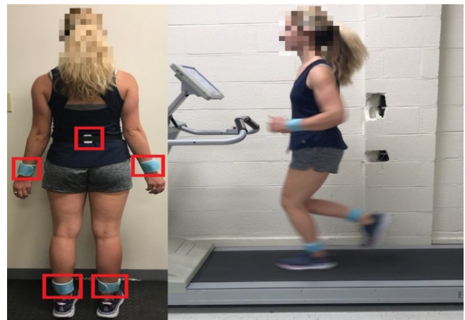
Fig. 2. Placement of inertial sensors on participant (Left) and data collection setting (Right)
