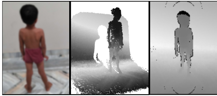
Fig. 1. (from left to right) (a) Back video of a child. (b) Point cloud data. (c) Depth image.
