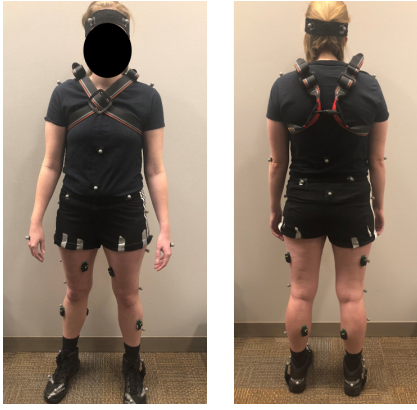
Fig. 1. One of the experiment subjects with sEMG/accelerometer sensors and motion capture markers.
