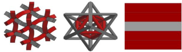
Fig. 3. We can see the different configurations used in this investigation, the red color represents Agilus 30 Clear and the gray color represents the VeroBlackPlus. In A we can see the configuration of CCF, CCF-HB. In B we can see configuration OTL-PC. In C we can see the MS configuration of the MM.
