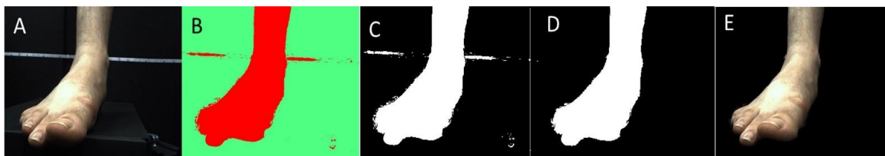
Fig. 2. Preprocessing of extracted frames from RGB video A) original frame, B) after ImageJ Trainable Weka Segmentation, C) after binarization in MATLAB, D) after removal of outliers, E) final segmented image.
