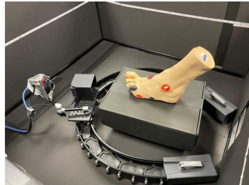
Fig. 1. RGB and Thermal Camera mounted on the Waterbird Track. The entire imaging stage is enclosed within the optical enclosure. A raised platform in the center serves as the platform for patients to place their foot upon for imaging.
