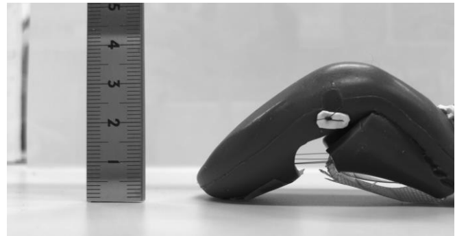
Figure 3. Test image of motion analysis of the artificial tongue deformation of artificial tongue unit using shape memory alloy fibers.
