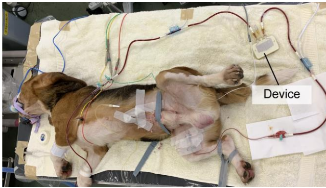
Figure 7 ex vivo experiment setup. Beagle(10.8 kg, Age 4.3, male)/IHFDC5/pressure gauge*2/polygraph system for pressure monitoring
