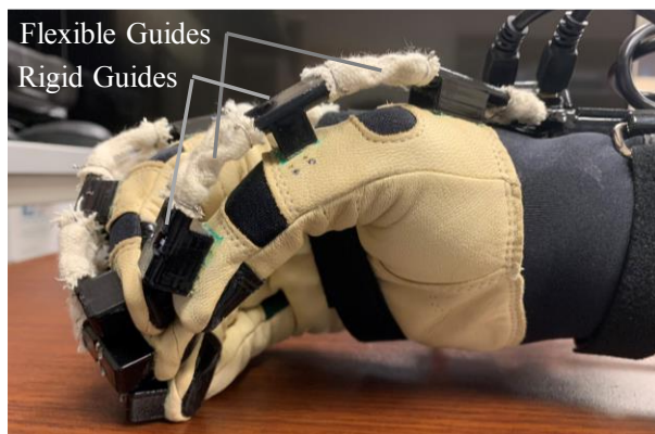
Fig. 2. Flexible guides prevent from cable buckling.
