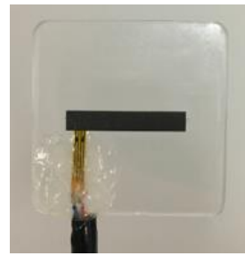
Fig 2. A sound transducer used in the experiments.
