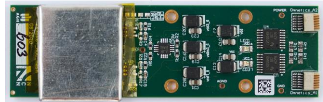
Figure 1. New design of an ASIC Board housing two Neurostim-3 chips (under metal shielding) and allowing usage of 128-channel Multi-Electrode Arrays (double connector on the backside)
