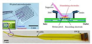
Figure 1. (Top) Fabricated 3D microelectrodes and *in-vitro* experimental set-up. (Bottom) Microelectrodes integrated with the PI cable and FPCB.
