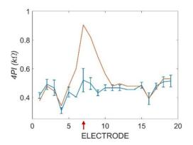
Figure 1. Four-point impedance measurements compared when blood was injected (orange line) into the 3D printed cochlea model, with the average measurements from the insertions. The red arrow indicates the point of blood injection into the model corresponding to the electrdoe array.
