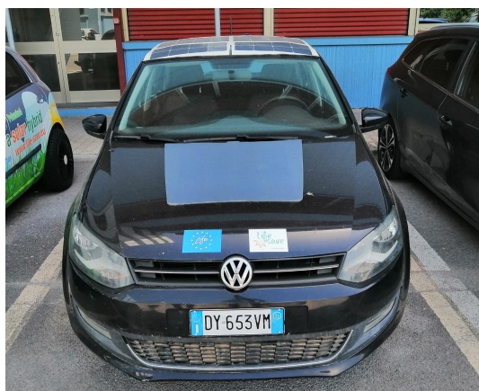
Fig. 3. The second prototype on VW Polo with solar panels on the roof
