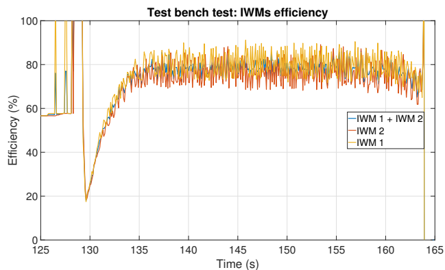
Fig. 10. Results on vehicle test bench: IWMs efficiency
