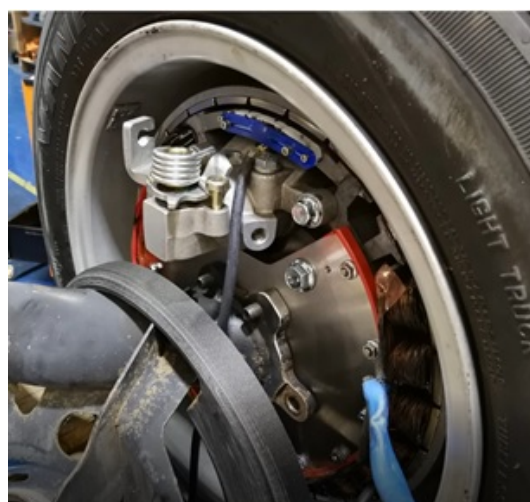
Fig. 5. Mecaprom designed In-Wheel Motors (IWMs) in the VW Polo Prototype
