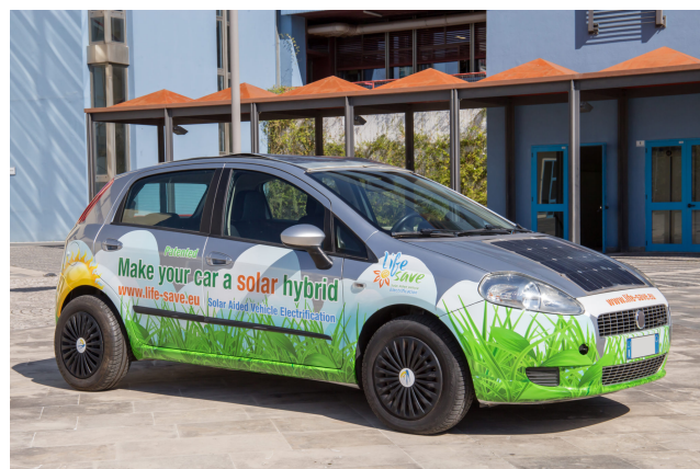
Fig. 2. The prototype of FIAT Grande Punto converted into solar hybrid
